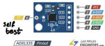
**VCC** supplies power to the module. Connect it to the 5V output of your Arduino.
